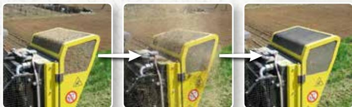
**RoboMAX** has been designed for working in dusty and hard situations. Moreover, it is equipped with an hydraulic reversible fan which can be controlled by remote control. It is possible to invert the rotation sense of the aspirating fan through the drive placed on the remote; this allows to blow away all the dirt on the radiator grid that may settle during the work. Consequently, the most important advantage is the radiator efficiency that allows also fuel saving.
